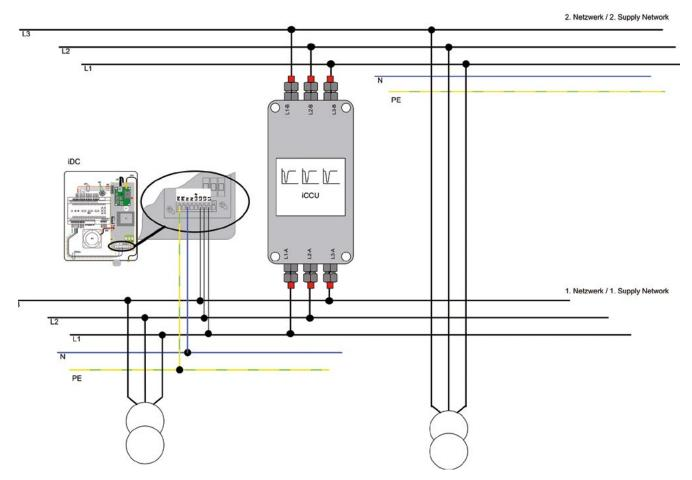
The iCCU can be used to couple the powerline signal into a further network.
